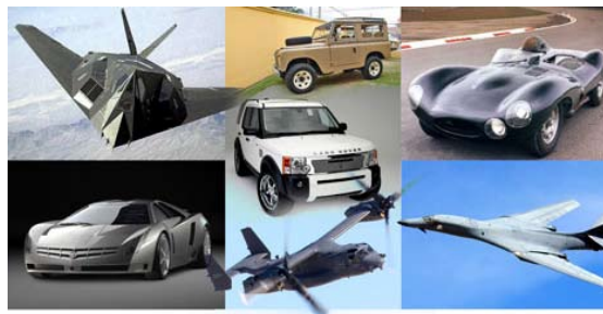
Picture 3. The three stages of surface continuity found in man-made products (left: positional , middle: tangent , right: curvature )
