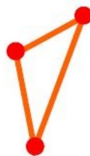
Picture 10. Triangle formed from three points: handle bar, seat and footrest on dirt/off-road motorcycles
