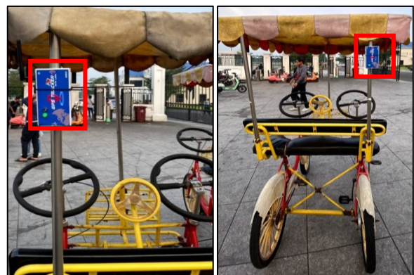
Figure 6. Installation of GPS Tracking 2 LoRa Node.
