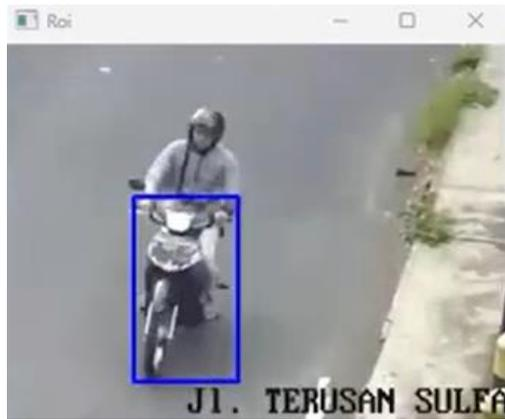
Figure 4. Detected Two-wheeled Vehicles using YOLOv5
